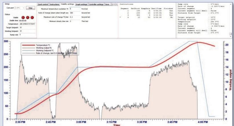
The brain of the furnace is the PID controller, a small box with led display, few buttons and a maze of menus and settings. The PID controller can be a challenge to use and it may lack crucial features. Omega Temp is a software that runs on a Windows based PC, connects to your furnace and to the PID controller in the furnace. Omega temp adds those missing elements and makes it easy to operate your furnace with few clicks of a mouse.
