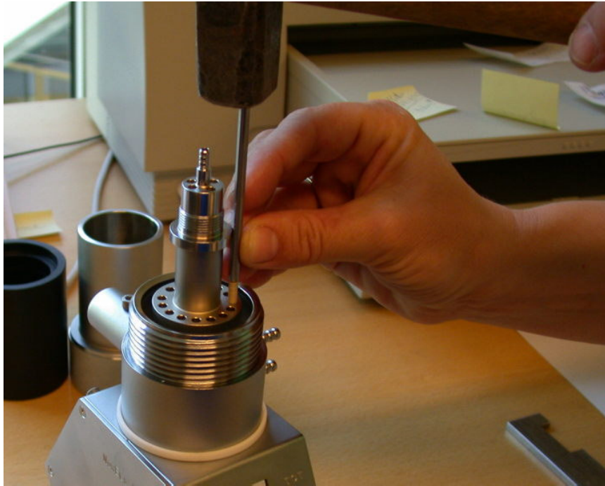
Figure 1-4. Hold the tool firmly, with the faceted side inwards, and hammer the assembly patiently all the way down.
