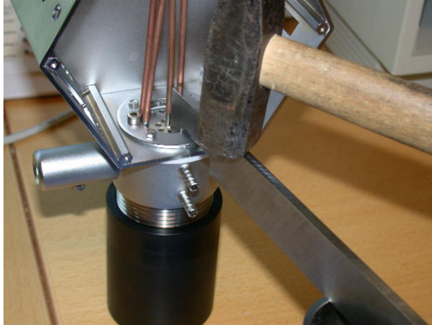
Figure 1-3. Illustration of how the flat steel tool can be supported on a metal object (lower right corner of the picture) instead of being hand-supported.
