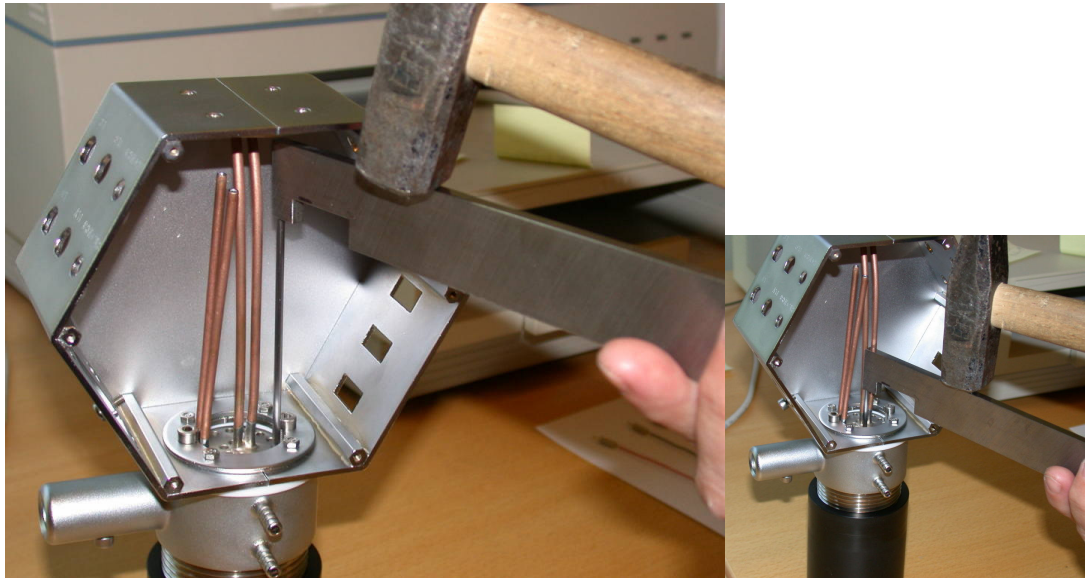
Figure 1-2. Hammer out the old PEEK (after wire has been removed). Left: outer ring feedthroughs. Right: Inner ring (pedestal) feedthrough.
