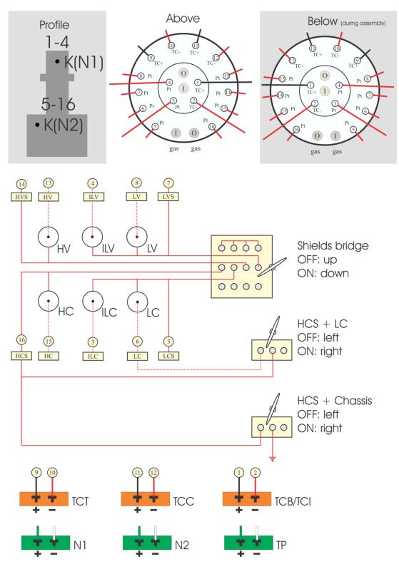
Wiring for ProboStat with Base Unit Heating
