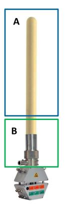
Area A is inside a furnace, and will radiate heat down to area B. The amount is different for each setup. Care must be taken not to overheat the region B. If the temperature is too low in the neck region B, consider using external means such as insulation or external heaters to increase the temperature in the neck.
