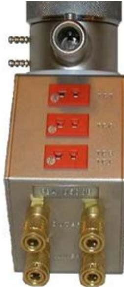
Fig. 19. Thermocouple sockets for S-type base unit. Fig. 20. Thermocouple sockets for K-type base unit.
