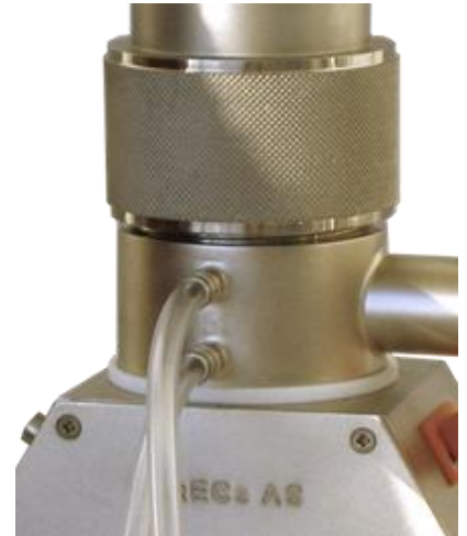
Fig. 29. Cooling water connected.
