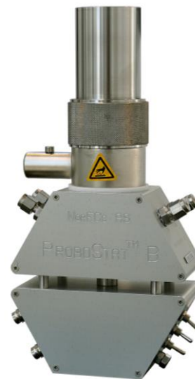
Fig. 3: SS bulkheads mounted on top part of splitted hexagon.
