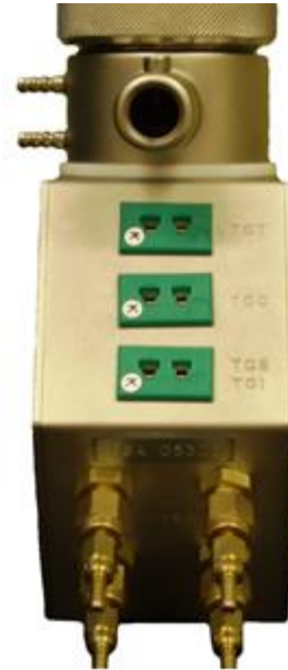
Fig. 19. Thermocouple sockets for S-type base unit. Fig. 20. Thermocouple sockets for K-type base unit.
