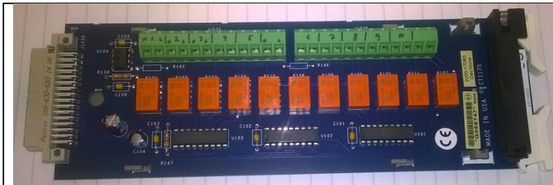
Channels as marked, 1 to 5 on left bank, 6 to 10 on right bank.
